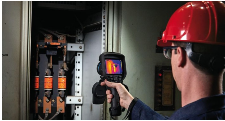
Thermographic infrared heat scanning
